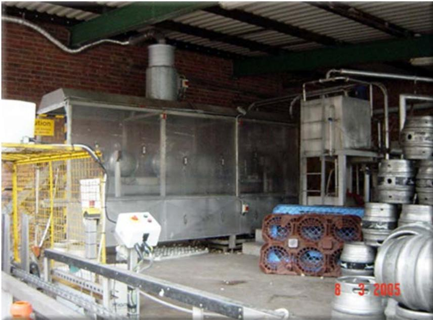
At Elgood's Brewery at Wisbech Cambridge the water is very hard with 330mg of Calcium and severe scaling was experienced particularly in the cask washer and also in the Angeleary Heater.
