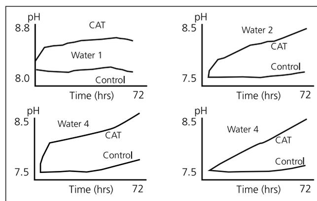
The same four synthetic waters were tested and spinners of copper (considered to be material that was inert – e.g a control), zinc (to represent a material that will be corroding fairly rapidly), and Colloid-A-Tron alloy were used. The pH was monitored continuously and a typical example of the change in pH over time is also shown in Fig.5.
