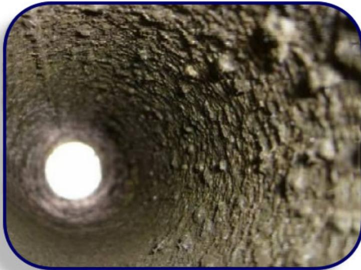
Scale formation inside compressors is caused by the deposition of calcium carbonate from hard water that is used to cool the compressor.
