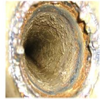
6 months of MagCat treatment with over 70% scale removed
